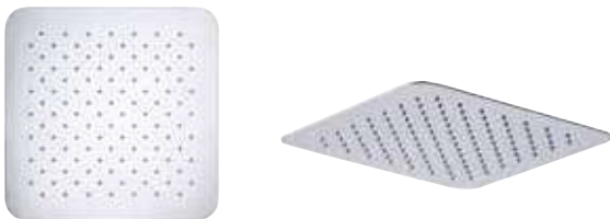
Square 300mm ceiling flush mounted stainless steel overhead shower 300(w) x 300mm(d) Minimum pressure 1.0bar
